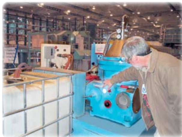
Vought process engineer Robert Nixon checks a centrifuge that performs periodic cleaning of four of Vought’s flumes.
