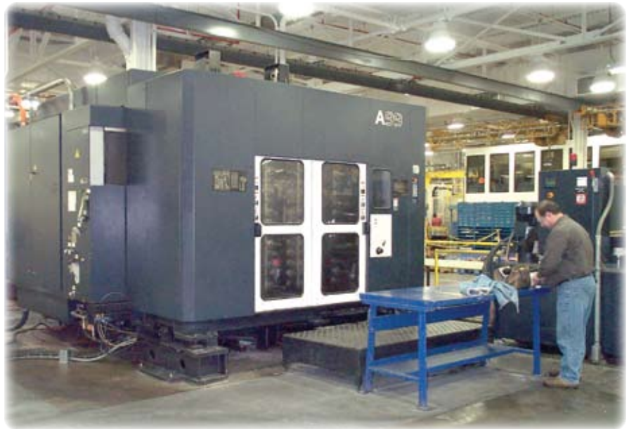
This Makino A99 horizontal machining center is used for high-speed machining of small parts at Vought Aircraft Industries Inc.
