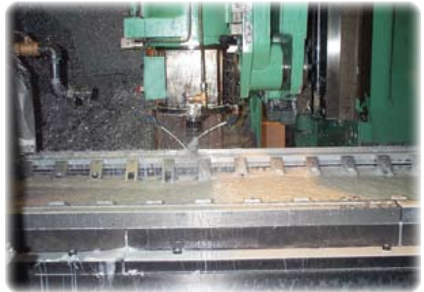
An Ingersoll spar mill is used to machine a stringer, using Houghton International's Hocut 795-B coolant technology.
