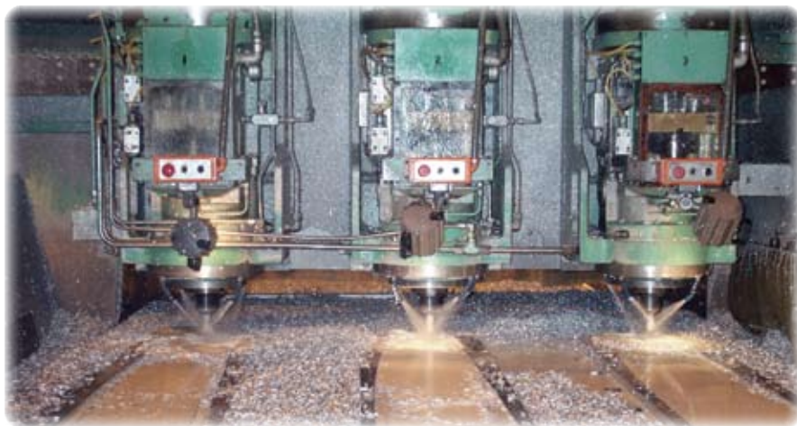
An aircraft bulkhead on a 3-spindle, five-axis Cincinnati gantry, during the machining process
