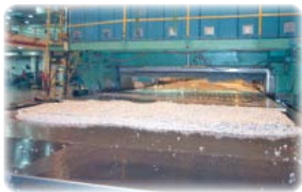
A two-spindle, three-axis Cincinnati skin mill, machining an upper wing skin section
