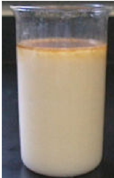
Moderate Recirculation Oil Breakout
