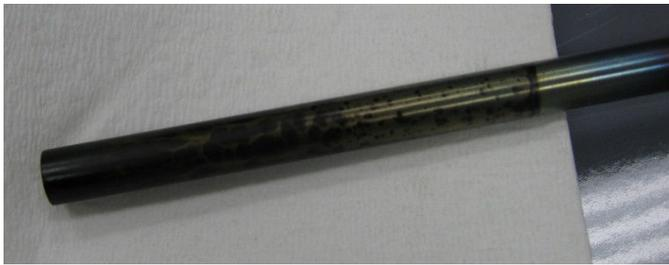
Figure 8. Stained probe from quenching severely oxidized quench oil.
