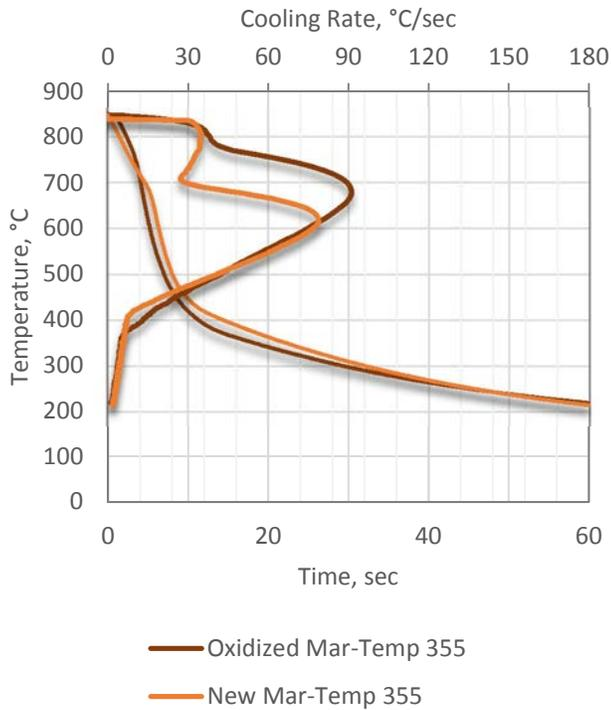
Figure 7. Severely oxidized oil showing change in cooling curve behavior.
