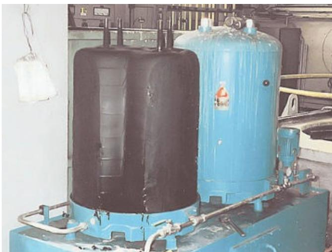
Figure 13. Typical high capacity filtration system designed for high capacity dirt loading and fine filtration.
