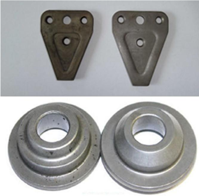
Figure 3. Parts before and after filtration showing an improvement in part appearance.
