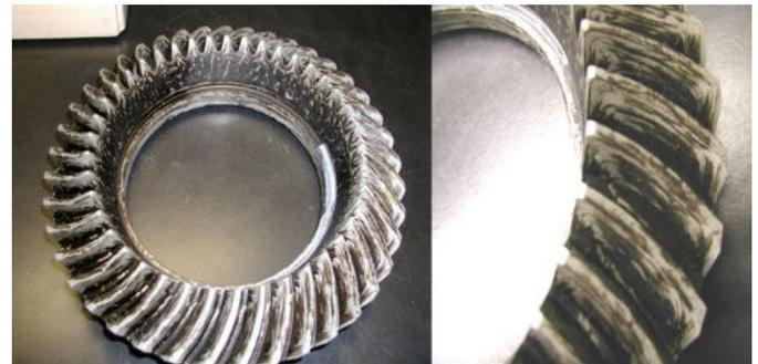
*Figure 1. Deposits on ring gears due to severely degraded quench oil.*
