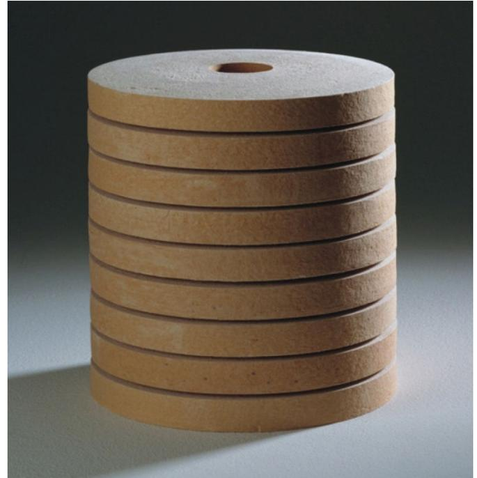
Figure 6. Deep Filtration Element used for cleaning quench oils to 3  $\mu\text{m}$  absolute and 0.8  $\mu\text{m}$  nominal. This means that 98.5% of all particles greater than 3  $\mu\text{m}$  and 50% of all solid particles greater than 0.8 $\mu\text{m}$ .
